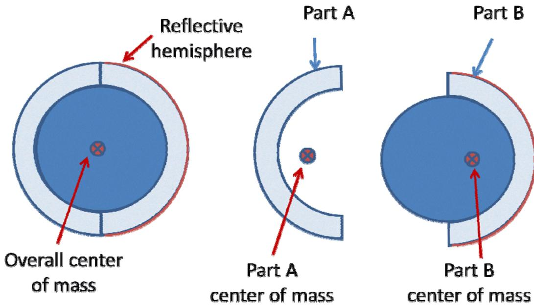
Fig. 5. BLITS Mechanical Failure Hypothesis
